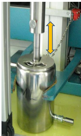
Picture 6 (Shaft protection and cover interlock)
