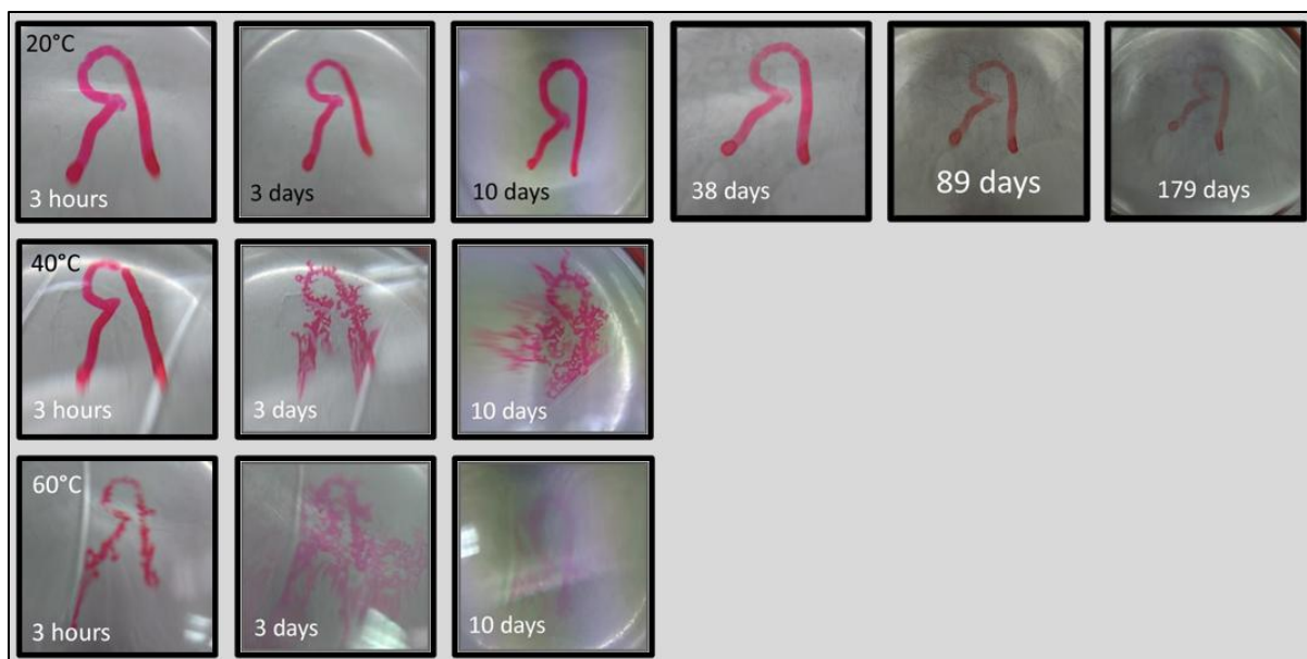
Figure 4: Photographs of the mark, at different timepoints, using 50% ethanol as the food simulant.
