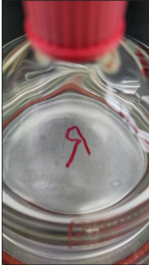
Figure 3: Illustration of the experimental setup. Because the “R”-mark is made on the reverse side of the transparent substrate, it appears mirrored. The side facing up is in contact with the simulant and is not marked.
